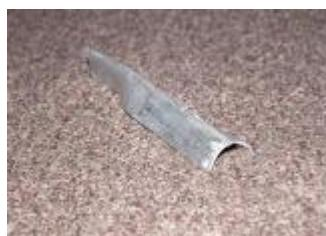
to avoid the risk mentioned above I use this piece of bent aluminium which is bent roughly to the same diameter of the outer bearing race.
