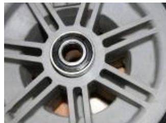
press the first bearing into the rim keeping the seal to the **OUTSIDE** like this.
