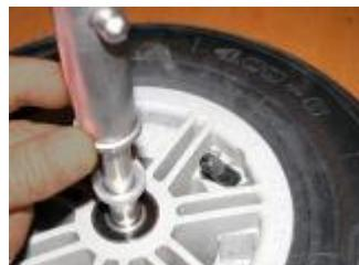
slide the stub axle AND WASHER into position
