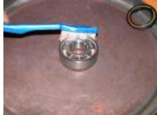
dip the toothbrush in the gas and start scrubbing, re-dip then re-scrub. Its a bit like brushing teeth only without the head.
