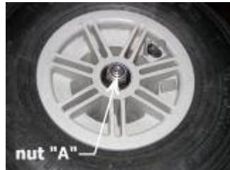
remove nut "A" from end of stub axle
