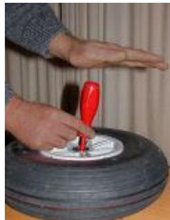
angle the screwdriver to catch the inside race of the bottom bearing and gently tap the bearing out. A little care is required as to not damage the bearing by excessive sideways force.
