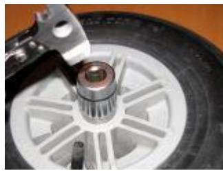
a socket with the same outer diameter as the bearing makes a good punch to press the bearing down to its seat. Be careful to ensure the bearing stays perfectly flat on the way in, If it starts going in on an angle you may damage the rim.
