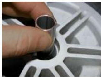
before fitting the second bearing, remember to put the spacer tube in. That's the bit of stainless tube that fall on the floor earlier that you weren't quite sure where it came from.
