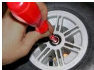
with all of the comprehensive range of screwdriver bits removed to line up the spacer tube ready for stub axle to be inserted. That screwdriver is proving itself to be very handy addition to your tool kit / utility belt)
