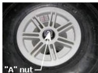
refasten "A" nut on the stub axle. Notice how the valve stem is now on the opposite side than the nut compared to how it was in the first photo of step 1. This puts the valve stem on the inside of the wheel, lessening the risk of valve stem extraction during close passing manoeuvres.
